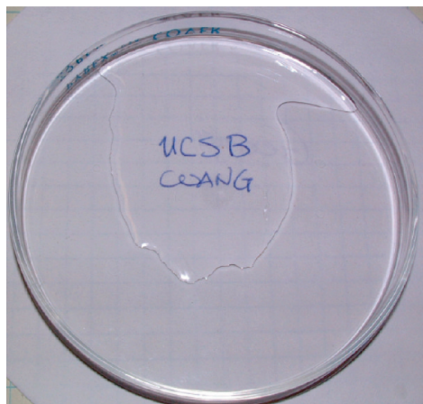
Figure 1. Photo of the sPP-EPR-sPP/mineral oil gel.
